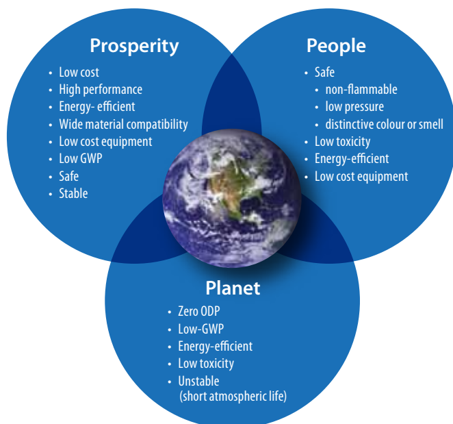
Figure 2: The properties of the perfect refrigerant mapped against the three dimensions of sustainability.
