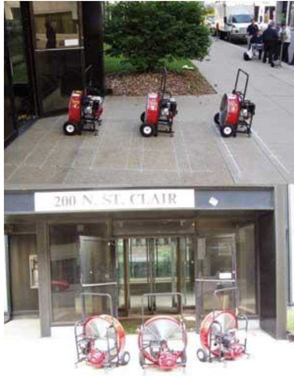
(1) Fans placed in a series (top) and fans placed side by side (bottom). (Photo courtesy of NISTIR 7412.)
